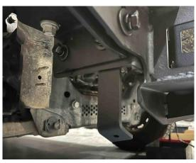
11. The Silver Bolt is used underneath the Chassis Rail Ends like shown.
