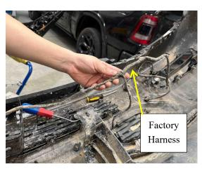
16. Remove the Factory Sensors from the Factory Bumper (IMPORTANT: the positions of the sensors on the factory bumper MUST be relocated to the same corresponding positions on the Supreme Bar). Setup the Sensor Chambers on the Supreme Bar as shown.
