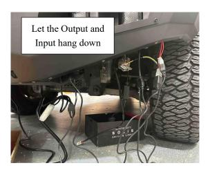
23. Fit and cable tie the RGB Harness Module to the Chassis of vehicle behind the Front Bar. Run the Single Thick Black Wire up to the engine bay next to the Battery then splice it to reveal the Yellow/Green Input Wire.
