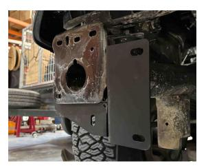
8. Fit the Cradle Bracket Piece onto the Recovery Brackets as shown below with the Bolts and Nut. Fit the Long Bolt (That was removed from step 4 back in securing the bracket) If the Long Bolt does not match the hole of the bracket, then cut a bigger hole to make it fit (use anti-rust on the hole that is cut). Refer to Step 9 Before beginning Step 8.
