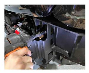
21. Have 2 people on each side supporting the Front Bar as you align it onto the front of the vehicle trying to make it as even and centered as possible. Make sure to leave a gap between 15-20mm. Once aligned secure the bar onto the Winch Cradle with the Brackets and bolts shown.
