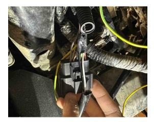
26. For both the Factory Head Light Sockets, extend the Signal Light Wire so it can reach the Yellow Wire of the Outer Cube Lights and connect them. NOTE: Blue wire does nothing.
