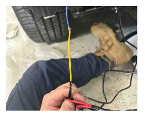
That should be all the lights (light bar and 4x cube lights), sensors and tech pack/radar all plugged in. Now bundle everything neatly together where you can and cable tie to have a tidy finish, no wires hanging or exposed and firmly secured.
