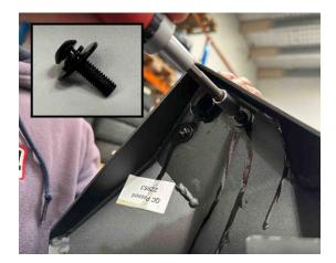
34. For Flare Extensions with the 5<sup>th</sup> and 6<sup>th</sup> sensor that will go on the flare extensions, the sides of the front bar will require cutting to allow for the shape of the sensor + plug to fit. Cut the Front Bar as shown on both sides. This will allow the sensors to fit like this.
