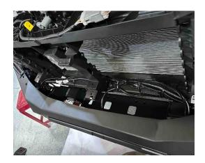
61. Once everything is reconnected and all wired up, you will need connect the RGB and HIGHBEAM harnesses to the vehicle's battery. Firstly, connect the Negative (black) wires with the metal ring to the earth which is on the passenger side of the engine bay next to the battery as shown and secure with a nut. Then connect the Positive (red) wires with the metal ring to the Positive Terminal of the vehicle's battery as shown and secure with a nut.
