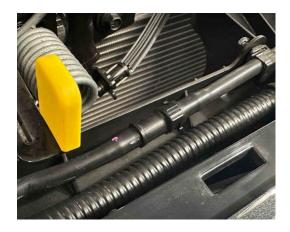
73. Put the plastic engine front cover back on and clip it into place with the factory clips.
