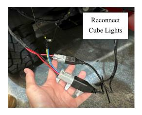
60. Connect the Yellow Wire from the Outer Cube Light Plugs to the Extended Signal Light Wires created back in Step (46) and (47). Then solder and wrap in electrical tape.
