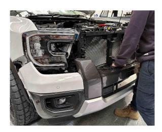
10. Remove the Plastic/Rubbery frame by removing any screws and clips, then remove the Foam Cover by removing the 2 clips holding it in place.
