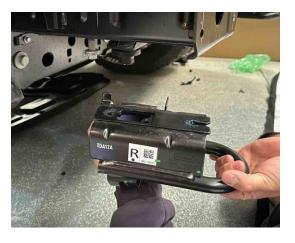
39. Pull off the rubber stopper as shown below, then put the 2 Square Intercooler Spacers (stacked together) in its place before putting the rubber stopper back on.
