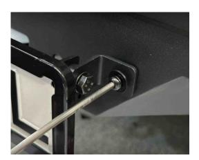
71. Re-fit the factory grille back onto the vehicle with the factory clips and screws/bolts.
