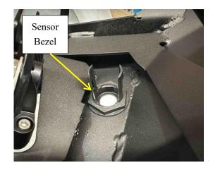
**NOTE:** Before fitting the 2 inner front factory sensors into the Bezel in the next step, the front bar must be fitted onto the vehicle first, because the sensor will get in the way of tightening the bracket for the Front Bar. So ONLY fit the 2 inner front sensors into the bezel AFTER the front bar is secured on. You can fit the other sensors first.
