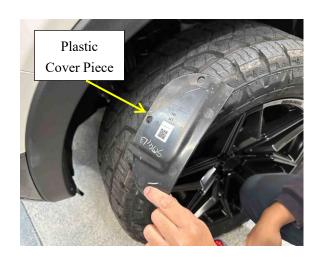
9. Gently lift the wheel arches on each side of the vehicle (CAREFUL not to break any clips) to reveal 2 more clips per side to be removed. Now the Front Bumper can be removed with a firm pull.
