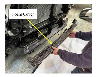
11. Remove the Tech Pack cover by removing the 2 clips carefully from each side, then unplug the Tech Pack and keep it aside somewhere safe.
