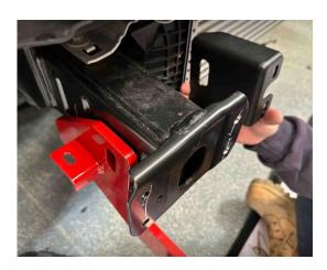
41. Loosely secure the assembled Recovery Point with the factory bolt underneath as shown. Use this long bolt provided to secure the side of the Recovery Point, but do not tighten completely as you will need to remove this long bolt in a later step.
