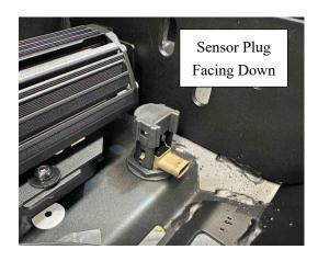
57. Re-plug in the Tech Pack Sensor and reconnect the factory headlight harness.
