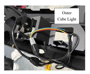
20. Now go to the outer cube lights and cut the blue wires (These are not needed) and then tape it neatly next to the yellow wire (**NOTE:** do NOT connect wires, just taped together so the blue wire is out of the way).
