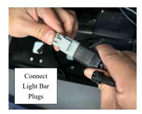
59. And connect all the RGB Lights to the RGB Harness like shown. There will be 6 plugs from the harness and 5 lights that need connecting (4 cube lights + 1 light bar) they can connect however you like and there will be 1 harness plug left over. Also reconnect the Cube Light Plugs together.
