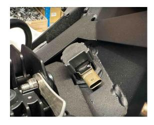
30. For vehicles NOT using the flare extensions and don't have a 5<sup>th</sup> and 6<sup>th</sup> sensor on the very sides of the vehicle then you can follow step (28) To install the Front Sensor Cover and the Sensor Bezel onto the very side sensor holes on the front bar and then instead of fitting the factory sensor into this Bezel, simply cover it up with the Sensor Cap.
