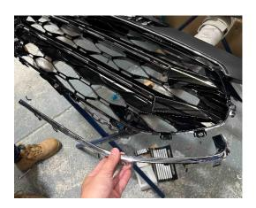
59. Next remove the lower black cross piece by unclipping the points shown here, it will take some force, you can opt to use a flat head screwdriver to assist, but be careful NOT to break any of these clips.
