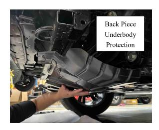
8. Remove this vertical metal piece on each side of the intercooler by removing the bolts. Discard the metal piece but keep the bolts.
