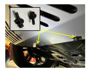
51. Then Fit the Frontal Bash Plate with the supreme word on, securing the 3 front points with the bolts and washers provided (But do not tighten yet).
