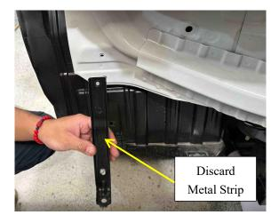
7. Remove the bottom 3-piece underbody protection by removing the bolts that hold them in place starting from the Front, then Middle and finally the Back piece. The 3 pieces can be discarded.
