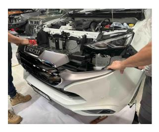
5. There is a vertical plastic piece near each headlight that needs removing. Firstly unclip the 2 clips holding it in place as shown below then the whole piece can be detached and discarded.
