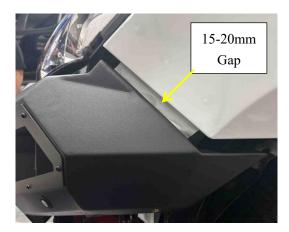
42. Secure the bar onto the vehicle using these brackets and bolts making sure not to tighten completely yet so you can make final adjustments to its alignment. Once you are happy with the alignment then you can tighten all the bolts to secure the bar onto the vehicle. You can tighten the bolts through the gap in the Front of the Bar like shown.
