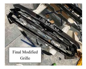
65. Fit the Newly Modified Grille back onto the vehicle, carefully resting behind the bar. There is a screw that needs to be secured on at the front (the factory screw kept when removing the grille), and also clips at the top.
