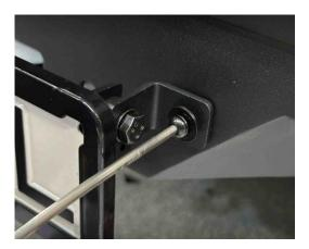
57. The Factory Grille requires modification to fit the Front Bar. Make sure to do these steps carefully as one mistake can ruin the grille. Firstly, unscrew the Grille from the Factory Bumper Bar
