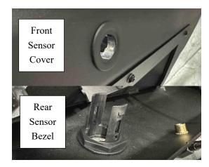
30. Fit the Factory Sensor into the prepared Sensor Bezel then push and clip in the Bezel Cap on top (make sure it is secured and clipped in). This is how to fit all sensors.
