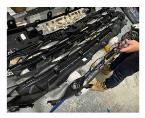
62. Cut along the points shown below to remove more of the lower part of the Factory Grille.
