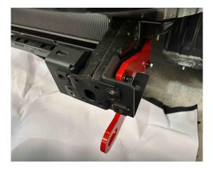
13. The 3<sup>rd</sup> Bolt will need to be shortened to about 45mm and used to secure the Rear Top Point of the Recoveries. This will require the Nut to secure. Don't tighten any of the bolts yet.
