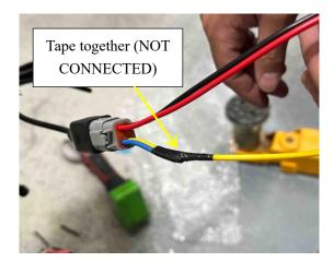
22. Now take the black wire from the Outer Cube Light and the black wire from the Inner Cube Light and join them together. Do the same for the red wires from the Outer and Inner Cube Lights joining them like so. Do this for both the right and left Cube Lights on the Front Bar.
