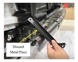
9. Remove the Metal Bumper Piece by removing the 4 Bolts. Then Remove the Plastic Condenser Frame which is held on by 4 clips.
