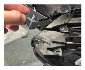
61. Cut the small attachment points indicated on the image below to remove the lower part of the Factory Grille.
