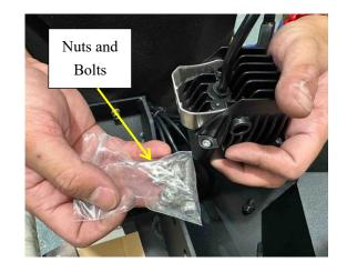
20. IMPORTANT: There are 2 different Cube Lights: the ones with 4 coloured wires attached (red, blue, yellow, and black) go on the outer side of the Front Bar (as shown in the image), while the ones with only black and red go on the inner part of the Front Bar. Once identified, place them in their correct positions and fit the Cube Lights onto the Front Bar like shown with the longer nuts and bolts.
