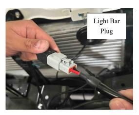
45. And connect all the RGB Lights to the RGB Harness like shown. There will be 6 plugs from the harness and 5 lights that need connecting (4 cube lights + 1 light bar) they can connect however you like and there will be 1 harness plug left over. Also reconnect the Cube Light Plugs together.
