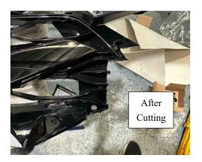
64. Finally re-fit the Black Cross Piece that was removed in Step (59) back onto the front of the Factory Grille by clipping it back on. The Final Modified Grille should look like this.
