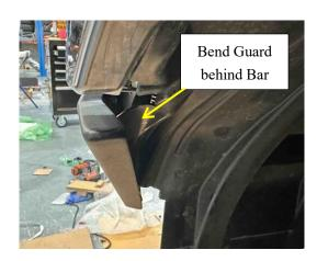
49. Fit the 2 Side Skid Plates under each side of the Front Bar using the remaining bolts as shown.
