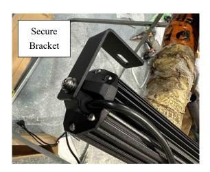
27. Place the Upper Grille onto the top of the Front Bar and put the light bar in position. Secure the Upper Grille and the Light Bar to the Front Bar using Bolt (F) from Step 25. Do this for both sides.
