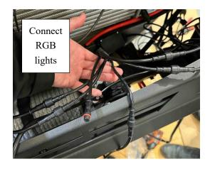
46. Cable tie all the Cube Light Wires neatly in a bundle to the Support Bar. Also Neatly cable tie all the Light Bar wires and Factory Harness to the Front Cross Bar in front of the intercooler.
