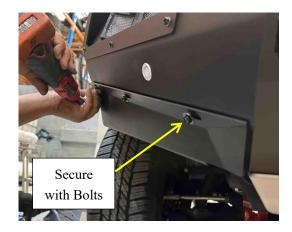
50. Fit the Factory Grille Bracket as shown and cable tie the temperature sensor back onto it.
