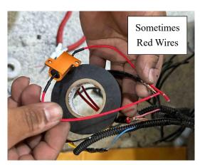
45. Connect the Light Bar Harness to the Light Bar Plug. Then connect all the RGB plugs from the 4x Cube Lights and the Light Bar to the RGB Harness plugs as shown. There will be 1 spare plug leftover.
