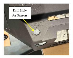
21. Unplug and remove the sensors from the Factory Front Bumper. IMPORTANT: note sensor positions on the Factory Front Bumper and its orientation, you must replicate this setup onto the Supreme Front Bar
