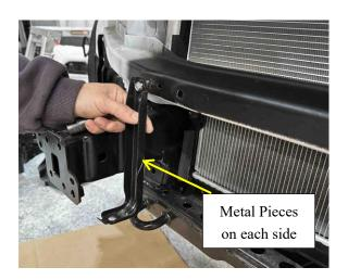
8. Further out there are 2 more vertical metal pieces that need to be removed. Then you need to unclip the temperature sensor in the middle.
