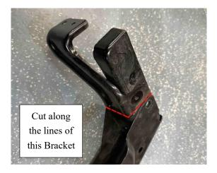
10. Keep those 2 brackets that are cut, you won't need the Metal Bumper Piece. Make sure to apply antirust or paint to the cut off ends to prevent rusting.
