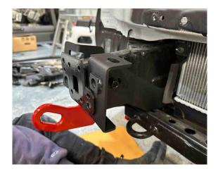
13. Setup the bolts as shown (A) (B) and (C). Then secure bolts (don't tighten yet) to the recovery points in the correct positions as shown. NOTE: Make sure the nut is the correct size fit, the wrong one will thread the bolt)
