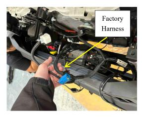
43. On the Factory Harness, locate the Blue Socket Head which is the Fog Light Socket. Cut the Blue Socket Head off to Expose the Black and Pink Wires. Connect that exposed Black Wire to the 2x Black Wires of the 2x Cube Lights on one side of the Bar. Then Connect the exposed Pink Wire to the 2x Red Wires of the same 2x Cube Lights. Do this for the Cube Lights on the other sides of the Bar.
