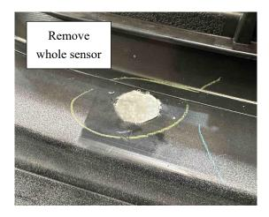
22. Modify the Factory Sensor Chamber by cutting off protruding plastic pieces so that it can squeeze into the Supreme Bar sensor holes, then fit them into the Supreme Bar. It should fit tightly.
