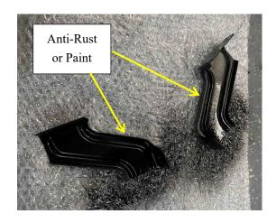
11. Refit the modified brackets that were cut off in the previous step back onto the vehicle supporting the headlights. Now also fit the additional headlight brackets provided on the sides as shown.
