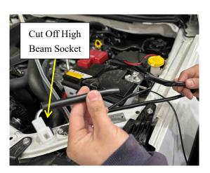
33. Connect the Black Wire from the Light Bar Harness to the Black Wire of the Head Light Socket from Step31. Then connect the White Wire from the Light Bar Harness to the Pink Wire of the Head Light Socket.
