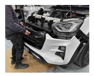
5. There is a vertical plastic piece near each headlight that needs removing. Firstly unclip the 2 clips holding it in place then the whole piece can be detached and discarded.
