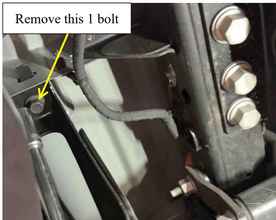
5. 1 Last Factory Bolt to be removed and kept is also near the other ones removed as shown. All factory bolts that are removed must be kept to reuse in fitting on the Electric Arm
