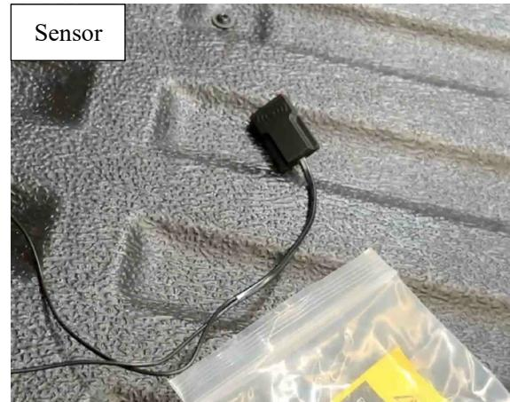
13. Stick the Sensor with the 3M tape in the position shown on the tail gate area above where the Electric Arm was fitted.
