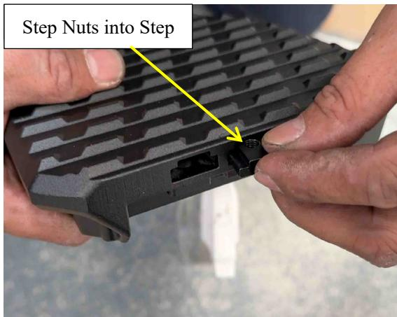
19. Put the Step on the Electric Arm then secure with the Step Bolts from underneath the Step
