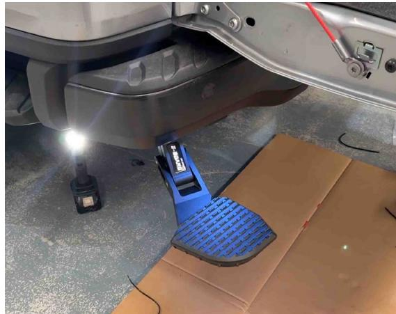
Make sure all bolts are tight, all cables and wiring are neatly bundled and tied.
