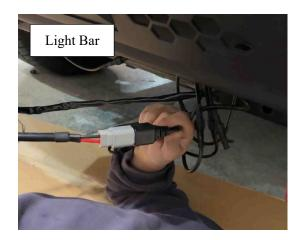
53. Now that all lights are connected and wired, neatly cable tie all wires and cables together and tuck into the bar.
