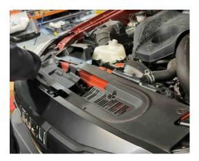
61. Run the Light Bar Harness Switch through the engine bay and into the driver's side to install the switch.
