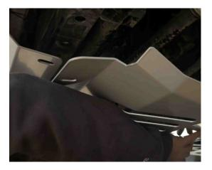
59. Connect and Secure both Front and Rear Bash Plates together using the Factory Bolts that were removed back in Step (5).
