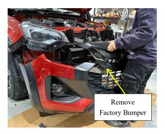
4. Remove the 2 Plastic Pieces on each side as shown, then remove the Metal Bumper Piece at the bottom by removing all the bolts.
