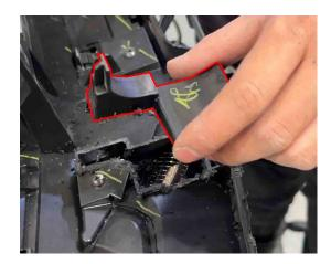
41. Refit the Grille back onto the vehicle using the factory clips
