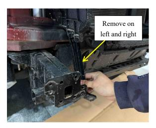
7. Then remove the Plastic Frame Piece then remove the 2 Metal Stripes on both sides.
