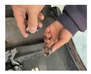
34. The Sensor Casing needs to be trimmed near the base where the Sensor Ring is to fit on the Front Bar.
