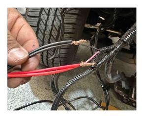
48. Take the Signal Light Wire we extended back in step (25) and connect it to the Yellow Wire of the Cube Light. Then Solder and Wrap in electrical tape any connections made.
