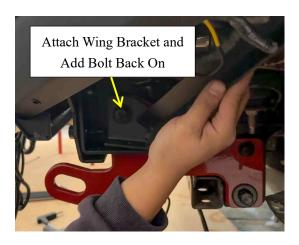
51. Now use the Bolt Setup from Step (49) To secure the Wing Support Bracket at its attachment points.
