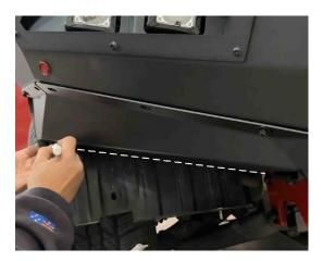
56. Take the Side Wing Cover off and Cut the Mud Guard where it is marked. Also Trim off the side of the Mud Guard where the Side of the Front Bar meets the Wheel Arch so that it can be tucked behind the Front Bar.
