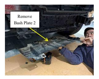
6. Remove the metal pieces shown for both sides of the vehicle.
