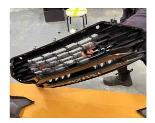
38. The Grille will need cutting to fit with the Front Bar. Cut along the lines like shown and keep the top part of the Grille.
