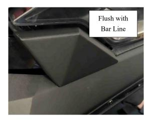
43. Have 2 people supporting the Front Bar as you align it to fit onto the vehicle. Make sure to leave a gap as shown between the vehicle and the bar.
