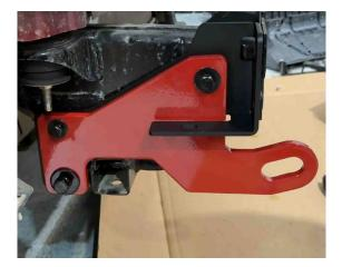
13. Sit the Winch Cradle in place on top of the Recoveries and secure the top outer points with the Factory Silver Bolts which were kept for both sides as shown.
