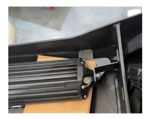
31. Remove the Factory Sensor/Fog light Harness from the Factory Bumper (Used later on)
